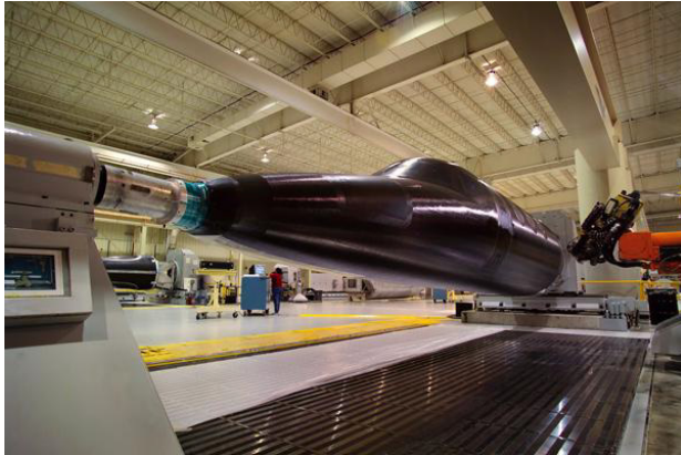
Figure 2. Fiber placement robot for airplane
