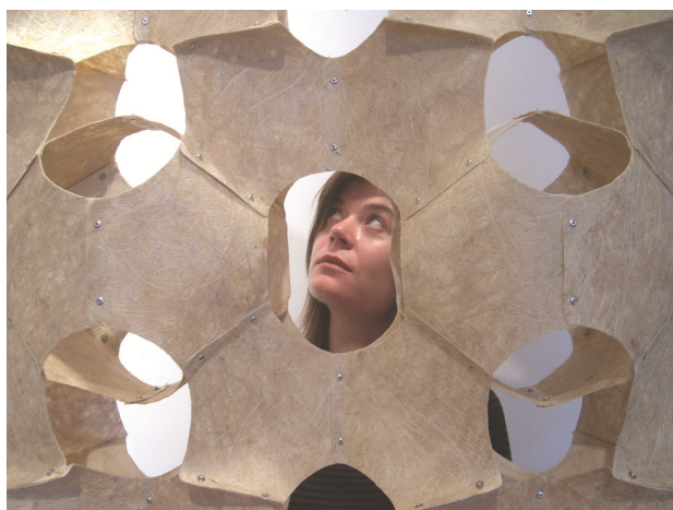
Figure 1. Green composite FiberWall made from sisal / linen fiber and soy resin
